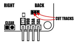
The two 10K pullups can be removed from the I2C bus by breaking the tracks between the 3 pads shown in the diagram above. Should you need to reconnect the 10K pullups at a later date this can be done by bridging the 3 pads with solder.
