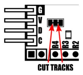
The two 10K pullups can be removed from the I2C bus by breaking the tracks between the 3 pads shown in the diagram above. Should you need to reconnect the 10K pullups at a later date this can be done by bridging the 3 pads with solder.
