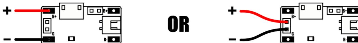
Connect your equipment to either power output solder pads, or the power out pin header.
