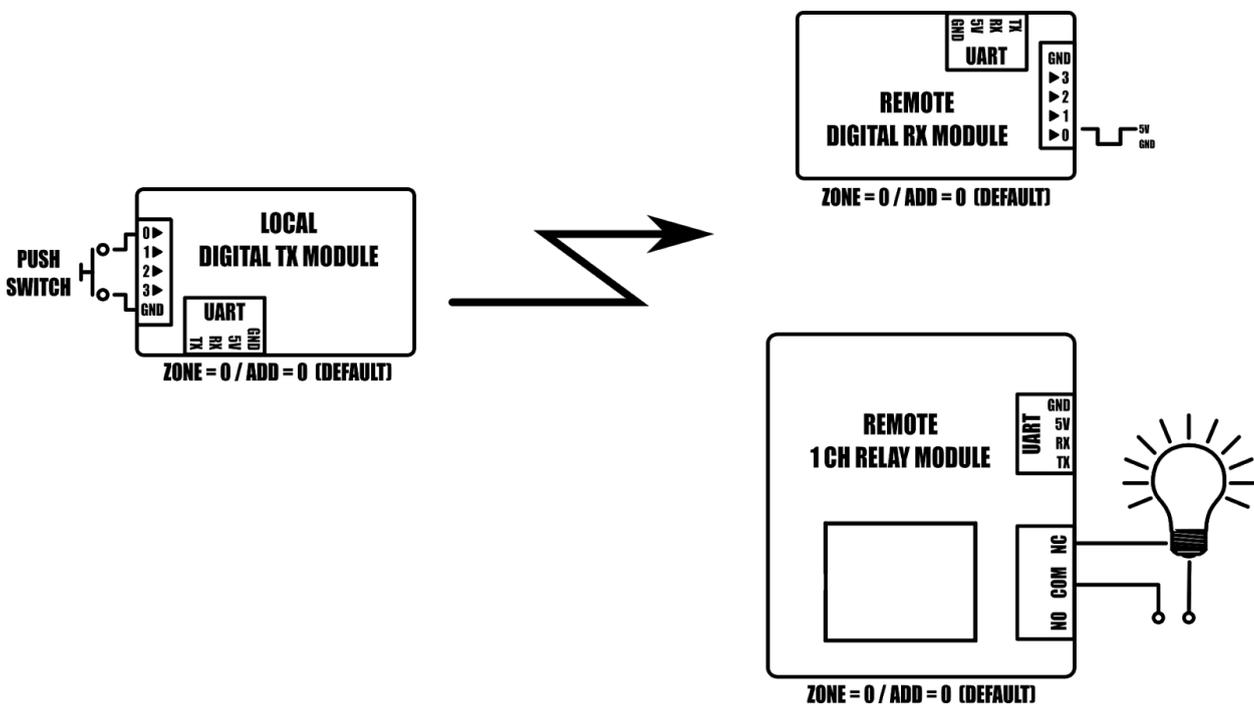
**Example: Controlling a remote digital pin and light from a push switch.**
