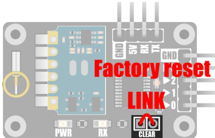
The module is capable of storing a number of user configuration settings in its non-volatile memory. This allows it to retain these settings even after power is removed. The two pads marked 'CLEAR' provide a means of restoring the module back to its original factory default settings. Should you wish to reset the module, connect power to the module whilst shorting the two pads together.
