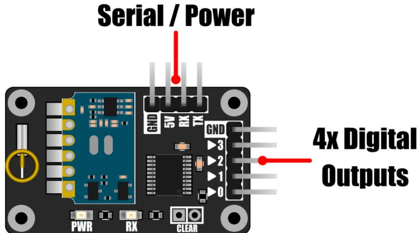
The SmartRFy digital Rx module provides a set of 4 digital output pins which can be remotely controlled by other SmartRFy modules. In particular when coupled with the digital Tx module (HCMODU0143) each pin on the Rx module will mimic the state of the 4 digital input pins on the Tx module without needing any configuration.
