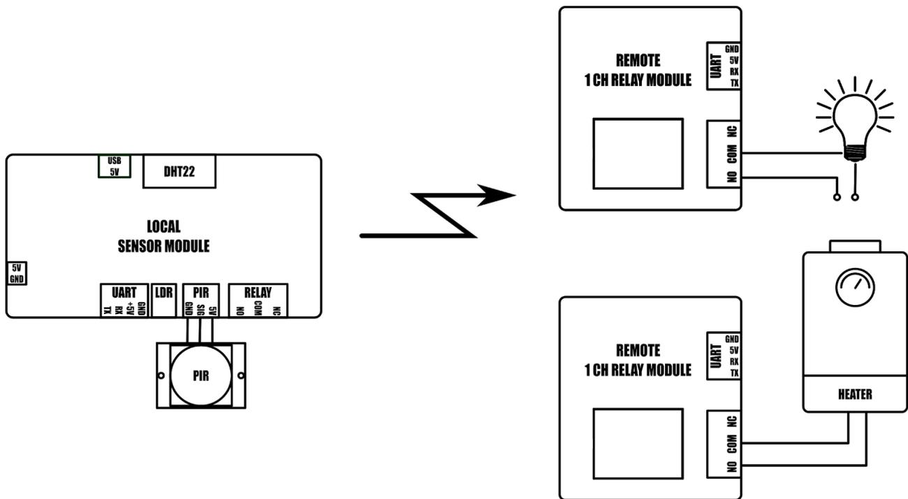
**Example: Remote 1CH relay module configured to turn on light when local modules' PIR is triggered and second remote relay module is configured to control a heating device based on local modules' temperature sensor readings.**
